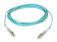
Fiber Optic Patch Cord, OM3, LC/LC duplex, 1.8 mm LSZH & OFNR, 60 m, aqua
